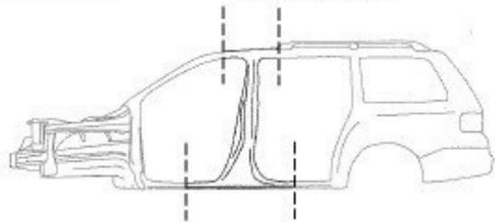
Standard Post Cut = 6 inches both directions at top post, halfway through each bottom door opening.
