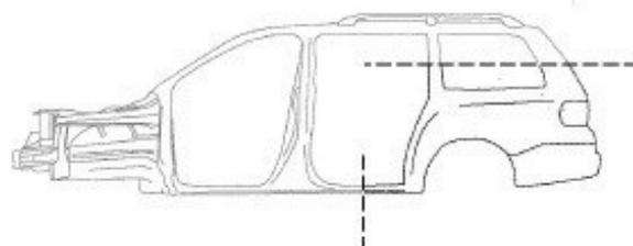
Standard 1/4 Panel Cut = Halfway down the sail panel and halfway through each bottom door opening.
